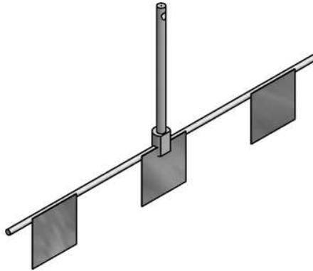
**Figur 3:** The torsion pendulum
