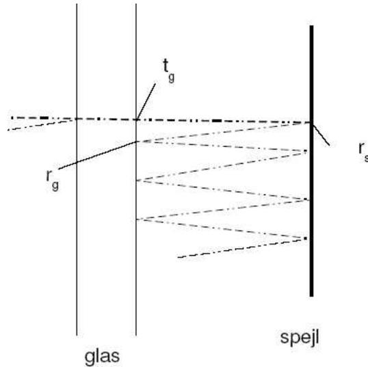
**Figur 9:** Reflections between the glass and mirror (spejl)
