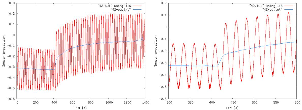
**Figure 7:** Turn-on of the source-laser with equilibrium curves
